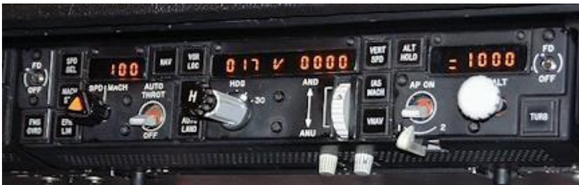
MD80 DIGITAL FLIGHT GUIDANCE SYSTEM (DFGS) CONTROL PANEL
